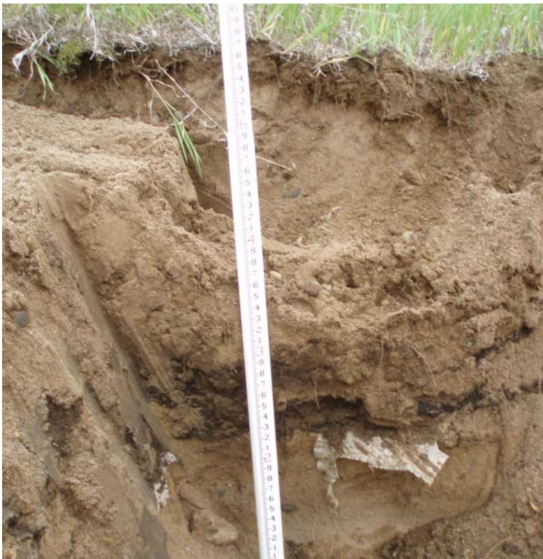
Photo 6 Former Lagoon Liner at SOC3-TT2
