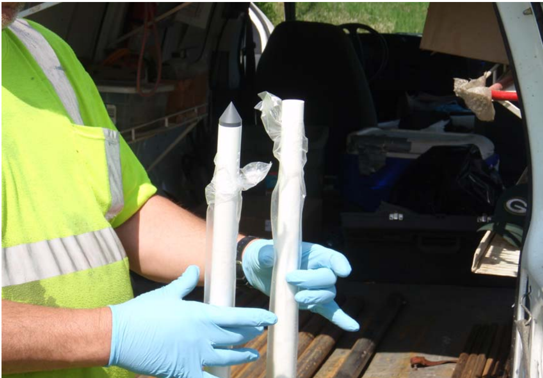
Photo 16 1" PVC screen and drive point
