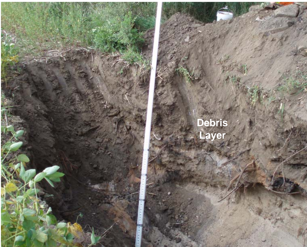
Photo 2 Test trench SOC4-TT9, debris encountered.
