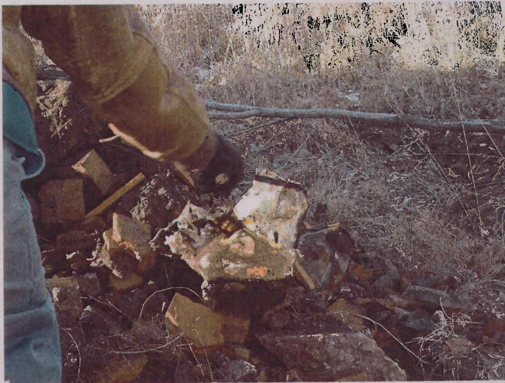
Wastewater Treatment Plant Area by Power Plant A. View of debris removed from test pit WWTP-TP-12 which included brick, slag, metal, tar, transite board, and electrical components.
