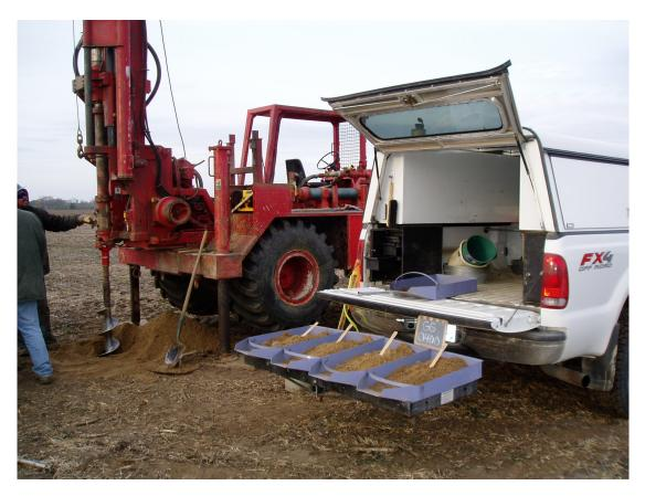
For the photographs, each pan containing a 5-foot sample was marked to indicate from what depth interval it was collected. Each photograph also contains a label on a chalkboard indicating the test hole number. Photographs are organized electronically so that the filenames reflect the test hole number and the sampled interval (testholenumber fromdepth-todepth). Photographs are grouped into file folders/directories by alphabetical row.
