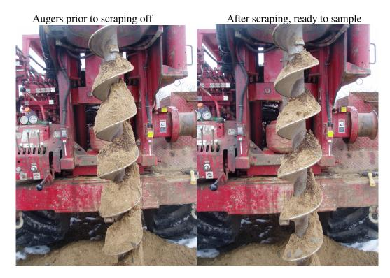
The more frequent the sampling (i.e., every five feet), the more accurate the stratigraphic control of each sample would be. However, sampling every five feet becomes very time consuming and therefore very costly. We proposed to sample the material encountered in each test hole in the following fashion:
